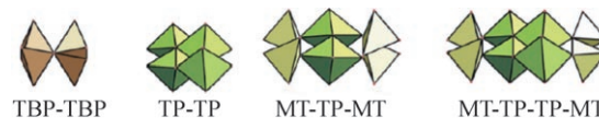
Figure 7. The four building units forming the double iron layers of the 2201- and 2212-type structures.
